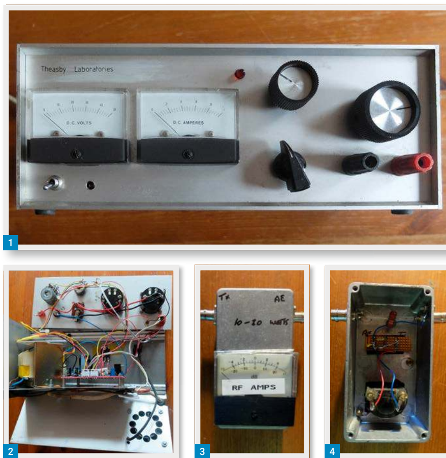
Fig. 1: PSU front panel before rebuilding. Fig. 2: The 'spatchcocked' unit open for access. Fig. 3: The RF ammeter seen from the front. Fig. 4: Internal view showing construction.
